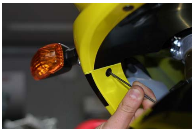
Figure 6: release the central clip of the plastic pin.
