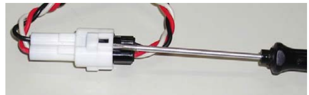
Figure 20: how to unplug a connector.
