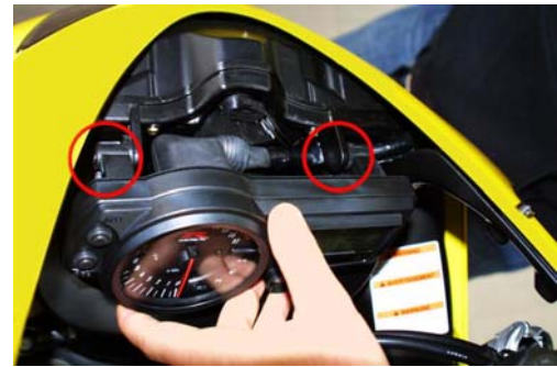
Figure 15: stock dash removal
