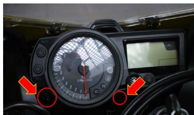
Figure 14: stock dash front screws position.
