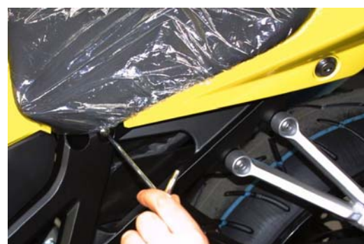
Figure 9: unscrew the bike screws
